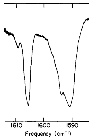
Figure 6. High-resolution infrared spectrum near 5°K of \text{BH}_3\text{CO}/\text{Ar} = 1/200 pyrolyzed.
